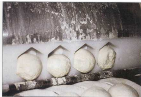
The bakery's new bialy machine automates "tagel" shaping and can produce about 270 dozen bialys in about 40 minutes.
