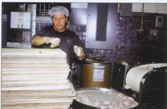
Joel Puma transfers shaped bagels to boards, where they proof for one hour, then spend an additional eight hours in the retarder.
